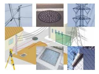
The narrow laser beam EDM not only can accurately measure the metope, angular point, ground, manhole covers etc. Light incident angle target, also can measure the high tension line or tree branches.
